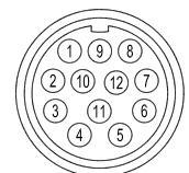
H connector (12 pin) - M23 CCW Hummel 7.410.000000 - 7.002.912.603 solder side view FV
