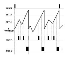
Output-4 continues counting after level of set-2 value. OUT-1 depends to OUT-2 and TOUT-2 should be selected as term. When count value rises above the level of the SET-1, OUT-1 is active and rises above level of the SET-2, OUT-2 is active. So count value will be fixed. Outputs and count value will be reset at the end of TOUT-2 period.
