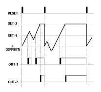
When count value rises above the level of the SeT-1, OUT-1 is active and rises above level of the SET-2, OUT-2 is active. So count value will be fixed. Even if encoder's pulse is at device without RESET, count value does not change but count value and outs will be reset.
