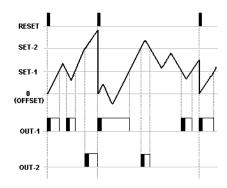
While count value is below level of Set-1, Out-1 is active and then Out-1 is inactive when on top of it. Out-2 is active when on top of SET-2 value and OUT-2 is inactive after reaching below the SET-2 value. Count value and outs will be reset when comes RESET.
