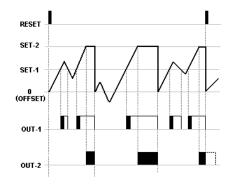
OUT-1 depends to OUT-2 and TOUT-2 should be selected as term. When count value rises above the level of the SET-1, OUT-1 is active and rises above level of the SET-2, OUT-2 is active. So count value will be fixed. Outputs and count value will be reset at the end of TOUT-2 period.
