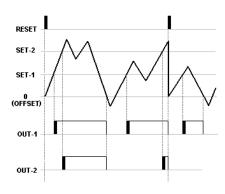
When count value rises above the level of the SET-1, OUT-1 is active and rises above level of the SET-2, OUT-2 is active. TOUT terms while selected HOLD, there is no outputs even to count value falls bottom level of SET values. Outputs will be reset when count value reaches zero (OFFSET), besides count value and outs will be reset when comes RESET.
