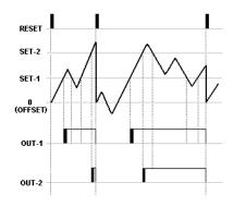
In this mode, when count value rises above the level of the SeT-1, OUT-1 is active and above the level of SET-2, OUT-2 is active. Relays will be active even goes down below the set values without RESET. Relays give outs during this time, if entered times for outs. Relays don't give outs until RESET.
