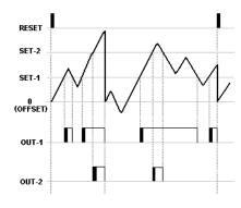
In this mode; when count value rises above the level of the SET-1, OUT-1 gives the out (so Relay-1 is ON). If TOUT-1 is selected (Time of Relay-1) HOLD, OUT-1 is active until count value falls bottom level of SET-1. When count value rises above the level of the SET-2, OUT-2 is give the out and If TOUT-2 is selected HOLD, OUT-2 is active until count value falls bottom level of SET-2. TOUT-1 and TOUT-2 are selected as term, OUT-1 and OUT-2 will active during this time.
