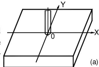
will feel it rather difficult to find out the datum zero mark when he/she want to continue the processing. If an SDS2 Series digital display box is used, the problem will have an easy resolution. SDS2 Series digital display box may keep the position of the datum zero mark of the working piece in memory.
