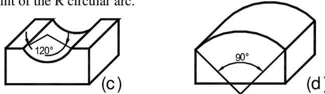
Note: When the arc to be processed in Planes XZ and YZ covers the 90° or the 270° position, for example, the one from 210° to 330° covers 270° in Fig.(c), and the other from 135° to 45° covers 90° in Fig. (d), end mill shall not be used.
