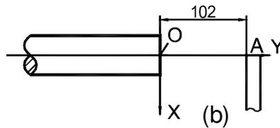
As shown in Fig. (a), the datum zero mark of the working piece is Point O, which is the absolute zero position.
