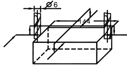
1) Move the tool along the direction of arrow and let it come to touch the one and the other edges of the working piece, then determine the center position.
