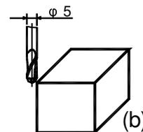
**2. At first, finish tool setting and return the boring ring scales on X- and Y- axes to zero.**
