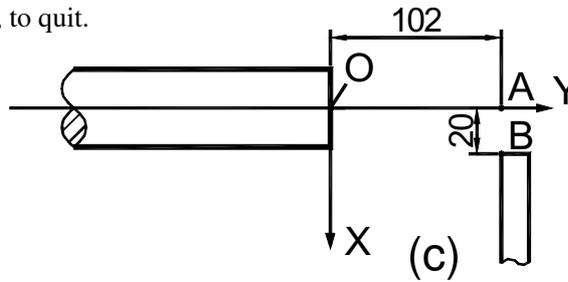
Searching the datum zero mark of the working point when turn on again power interruption or switching.
