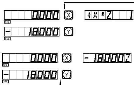
Move the machine tool to bring the displayed on X axis into zero, refer to the displayed value on Z axis and let the machine table rise or drop by the same value.
