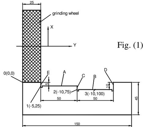
Reset, set the zero position in the absolute mode at the main reference of the working piece.
