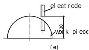
Move the electrode to the shown place in drawing (e).
