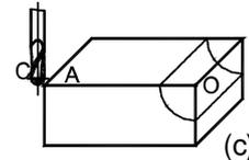
As shown in Fig. (c) when a circular arc milling tool is used, the circle center position is the position of Point O with respect to Point C on the tool.
