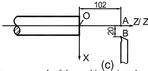
Searching the datum zero mark of the working point when turn on again power interruption or switching.
