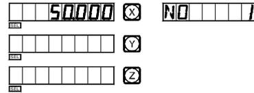
The display result for dividing the arc into 6 equal sections.
