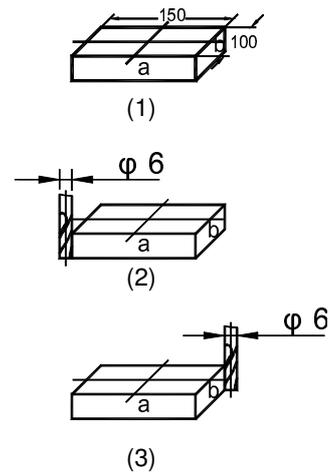
**Note: The tool diameter can be made only in the direction of X- or Y-direction.**
