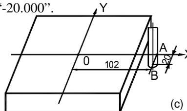
Searching the datum zero mark of the working point when turn on again power interruption or switching off.
