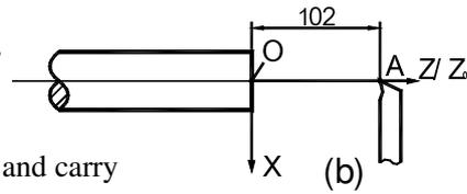
As shown in Fig. (a), the datum zero mark of the working piece is Point O, which is the absolute zero position.
