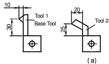
2. Ensure the other tool position relative to the base tool position, which is also the zero point of "ALE" coordinate system, as the figure (a) shows, the relative position of the second tool is:
