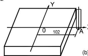
reference point A of the grating ruler. The digital display box will automatically track and carry out the datum zero mark tracking function.
