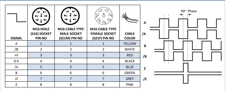
The table above shows the cable colors of the sensor output signals. If the control circuit is suitable in the Line Driver sensors of the not output signals (/A, /B, /Z) have to be added to the system. If it is not suitable /A, /B, /Z signal cables must be fixed as insulated separately. Don't forget that these edges have electricity too.
