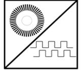
AWE 120 wire encoders convert linear motion into incremental digital pulses. Different stroke lengths from 300 mm to 2100 mm are available. Optionally other stroke lengths, resolutions, cable lengths and socket connectors can be requested.
