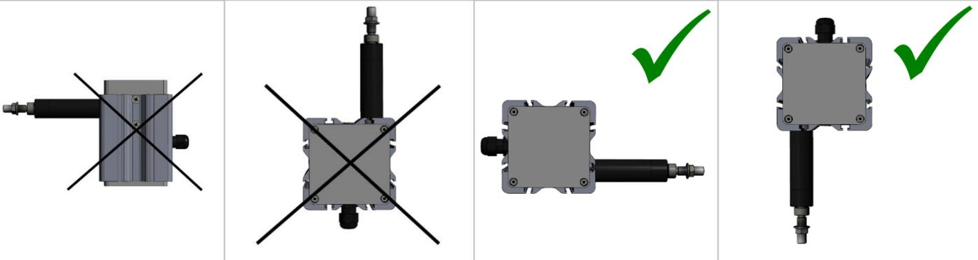
**3. If there is a trickle of water (like a rain), the wire outlet must not be a drip of water upstream. If needed please use guide rollers.**
