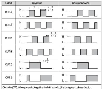
Counterclockwise (CCW): When you are looking at the shaft of the product, it is turning in a counterclockwise.
