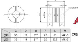
When coupling is combined in spin axis, The big combination err (Partial disposition, Declination) between spin axis and coupling may cause of shorten of life-time for encoder and coupling.
