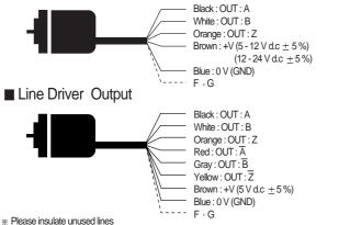
\* Metal case of encoder and Shield line must be ground connection.
