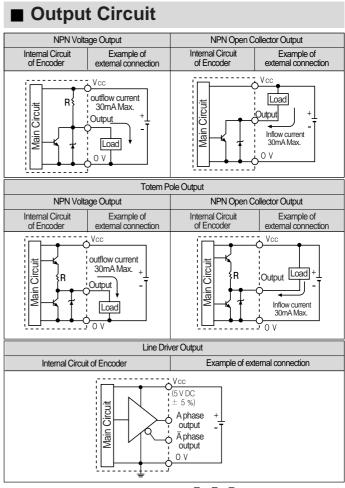
$\underline{X}$  The output circuit of A, B, Z phase (Line drive output A,  $\overline{A}$ , B,  $\overline{B}$ , Z,  $\overline{Z}$  phase) is same.
