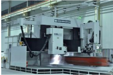
日本住友数控龙门平面磨床 SUMITOMO gantry CNC surface grinder from Japan
