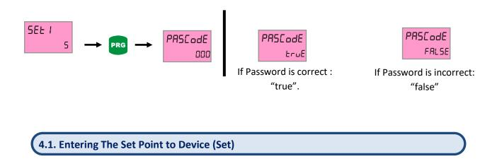
Menu is displayed firstly on the screen as prg button is pressed while operating mode. Menu of Set 2 is displayed while down button is pressed. The top row shows the name of the menu and bottom row also (yellow marked) selected value in menu content. Set 1, set 2 allows controlling to out1 and out2 relays.
