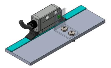
The magnet and Z reference sensor must be parallel to each other for the external Z reference signal.
