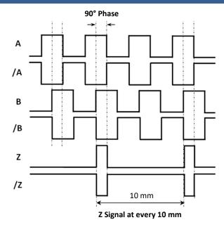
In the above table, the cable colors of sensors output signals are given. If the control circuit is suitable in the Line Driver, sensors of the not output signals (/A, /B, /Z) have to be added to the system. If it is not suitable /A, /B, /Z signal cables must be fixed as insulated separately. Don't forget that these edges have electricity too.
