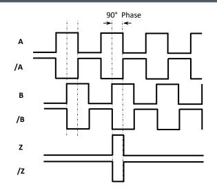
In the left tablet he cable colors of sensors output signals are given. If the control circuit is suitable in the Line Driver sensors of the not output signals (/A, /B, /Z) have to be added to the system. If it is not suitable /A, /B, /Z signal cables must be fixed as insulated separately. Don't forget that these edges have electricity too.
