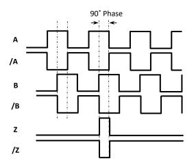
The table above shows the cable colors of the sensor output signals. If the control circuit is suitable in the Line Driver sensors of the not output signals (/A, /B, /Z) have to be added to the system. If it is not suitable /A, /B, /Z signal cables must be fixed as insulated separately. Don't forget that these edges have electricity too.
